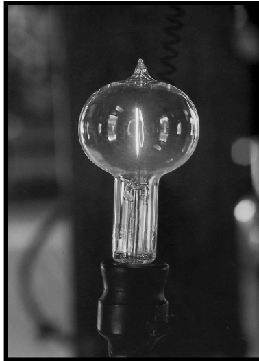
Fig. 1. The Edison's incandescence light bulb in 1882. (Courtesy of GE Company).
