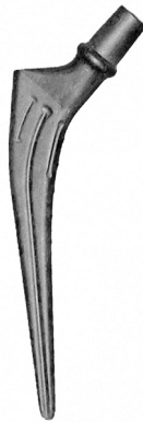
Fig. 1.4 Hip endoprosthesis stem, injection molded, chopped long fiber reinforced PEEK, fiber volume content 50% [M. Semadani, Ph.D. Thesis, ETH Zurich, 1999].
