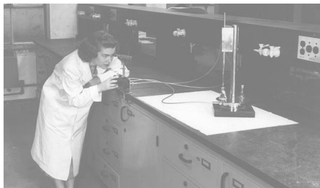
Fig. 5. Darleane Christian, Spring 1950 photo at Ames Laboratory, with remote apparatus for pipetting radioactive solutions.
